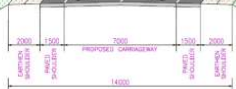
TYPICAL CROSS SECTION OF BRIDGE OF 2-LANE CARRIAGEWAY WITH FOOTPATH AND ITS APPROACHES FOR EMBANKMENT HEIGHT MORE THAN 3.0m (AS PER DRAFT CIRCULAR)
